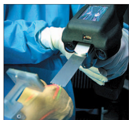
This is Trak Surgical's freehand, sensor-guided surgical saw.
