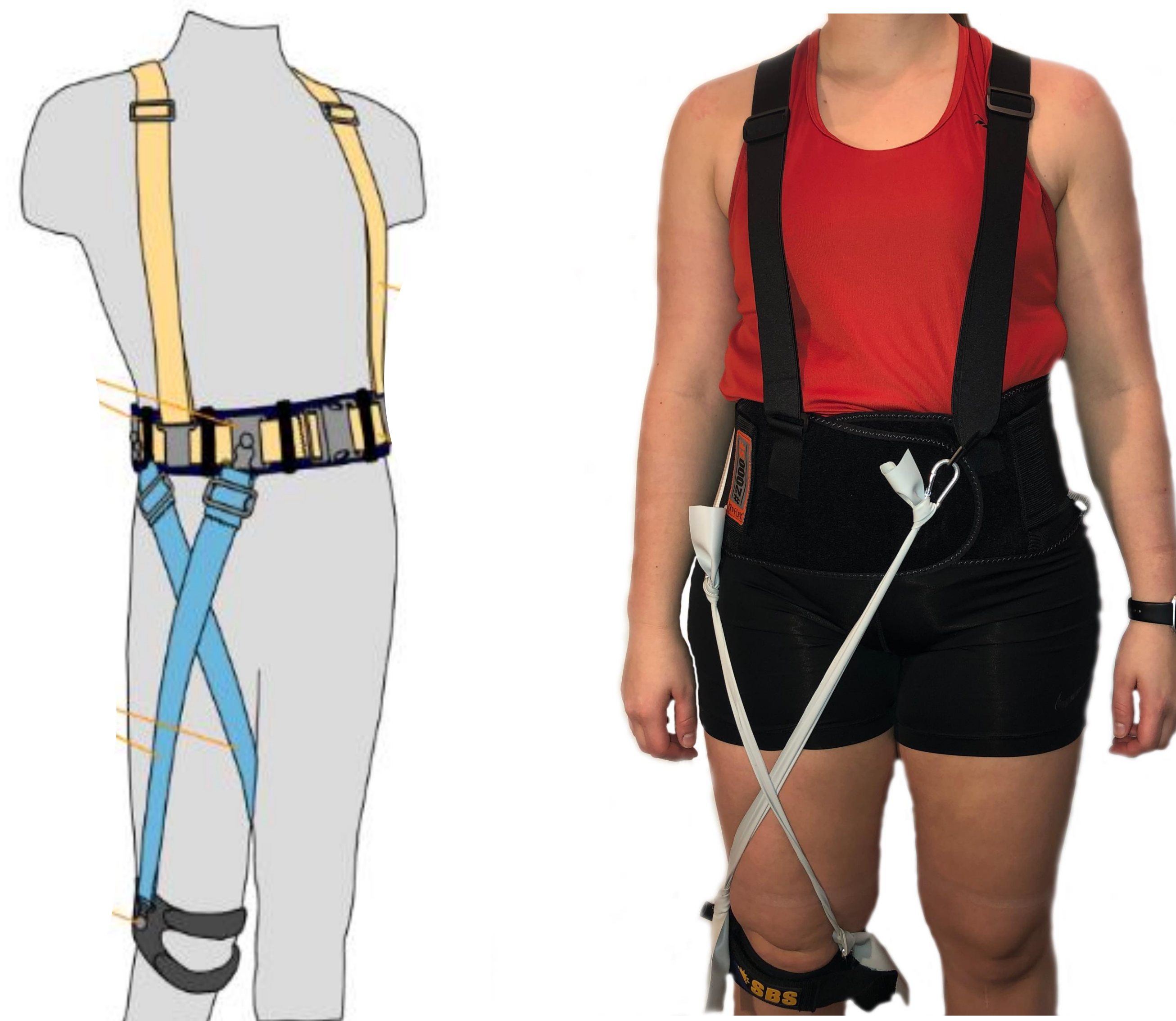
Figure 1: Example of a previous design (left) of a unilateral exoskeleton and the design of the proposed exoskeleton (right) [2].
