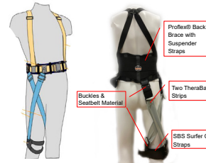
Figure 1: Example of a previous design (left) of a unilateral exoskeleton and the design of the proposed exoskeleton (right) [2]
